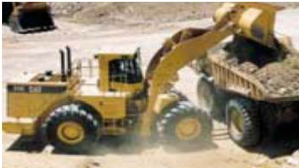
Fig.2.3 A Loader during loading on dump track.
