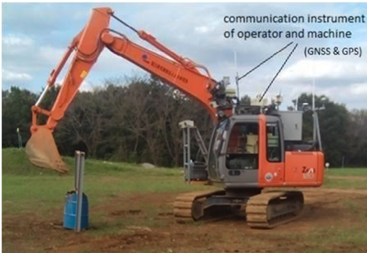
Fig.2.14 Unmanned construction machine in Japan.
