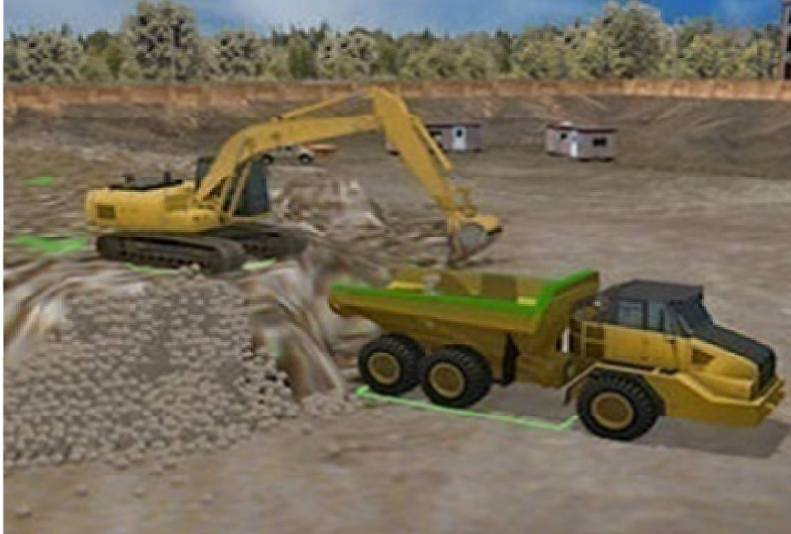
Fig.2.13 Excavator loading on the dump truck in the simulator in ERA at AMBTTC
