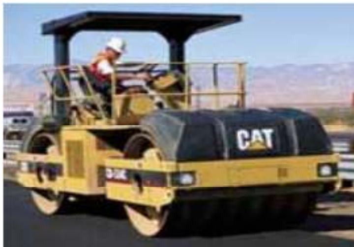
Fig.2.7 Asphalt Vibratory Compactors are designed for compaction and finishing of road surfaces.
