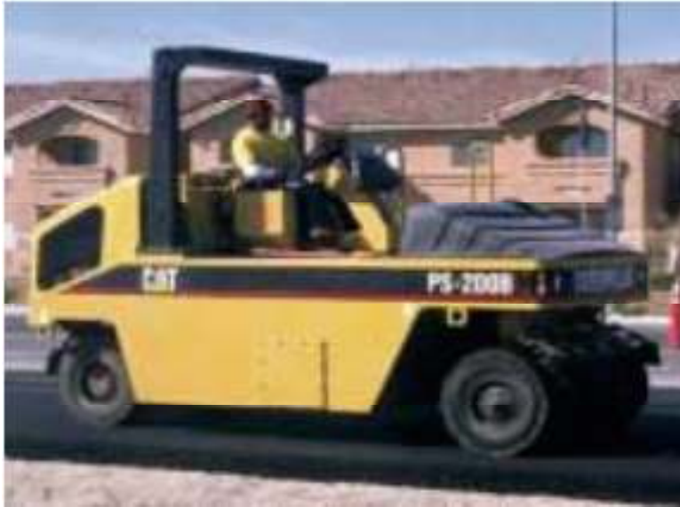
Fig.2.8 Pneumatic Asphalt Compactors are designed for compaction and finishing of road surfaces.
