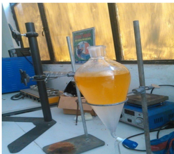
Figure 3.6 Oil into decanter for washing and layer formation
