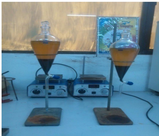
Figure 3.5 Oil into decanter and layer formation
