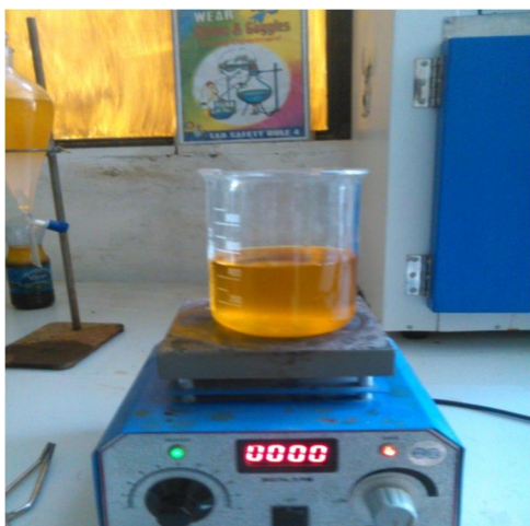
Figure 3.7 Heating and drying the biodiesel
