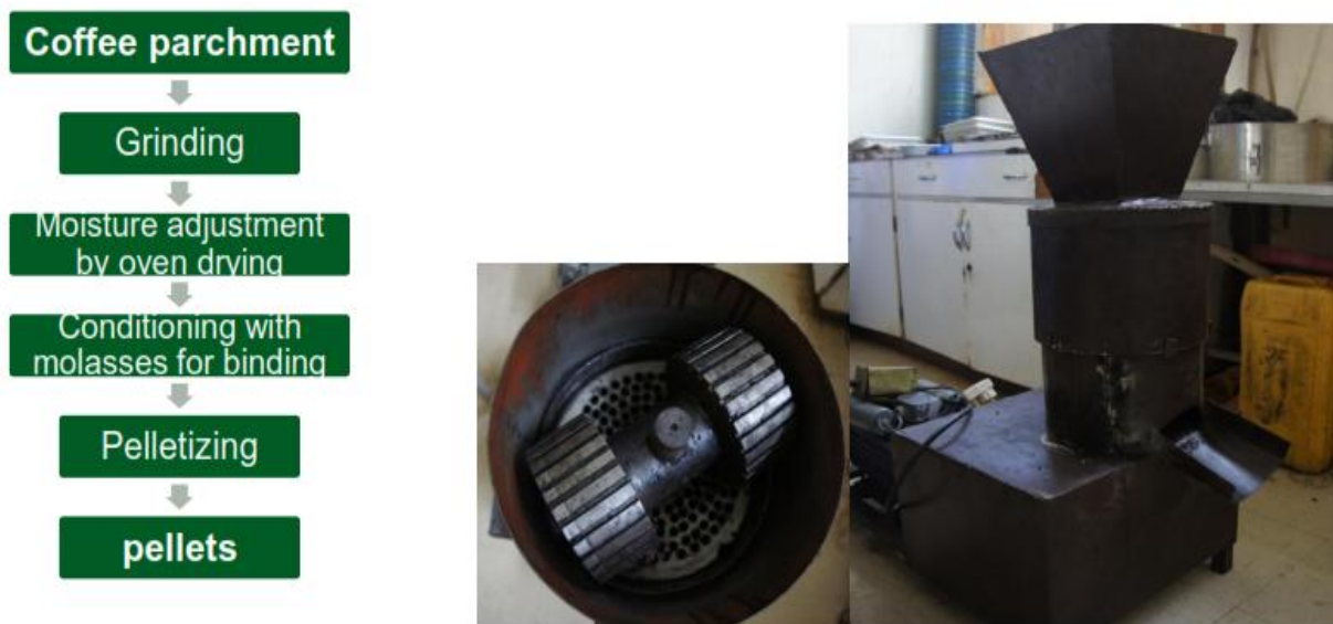
Figure 5 pellet formation phases from coffee parchment and pelletizing machine used
