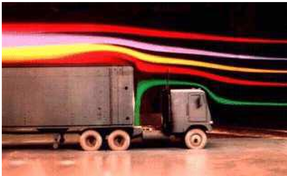
Figure 2.4. Flow over truck [48]
