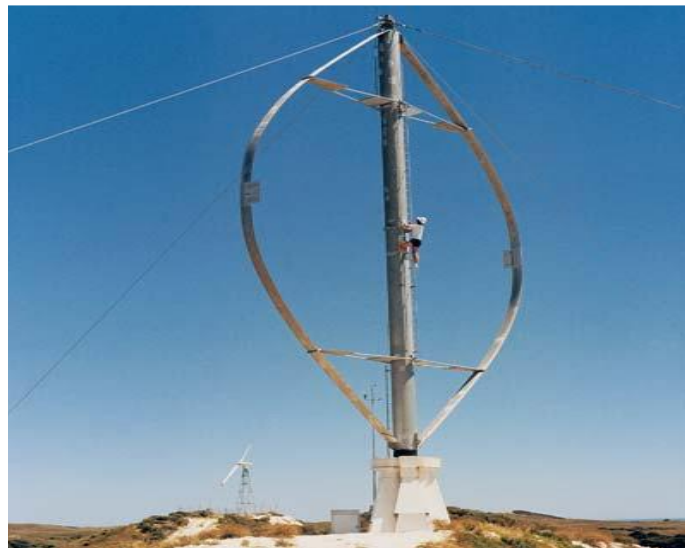
Figure 2.2. Vertical axis wind turbine (Gelma B, 2012)
