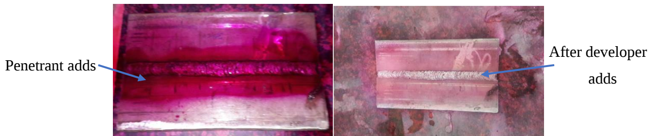
Figure 3.7 Treated sample when liquid penetrant is processed
