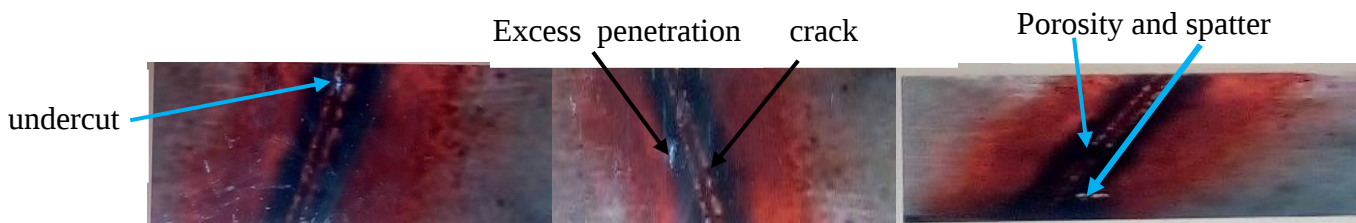
Figure 4.1 indetfication of defects
