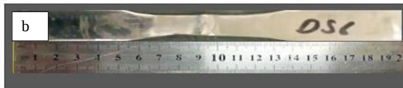
Figure 3.9 sample prepared for tensile strength from mild steel specimens.
