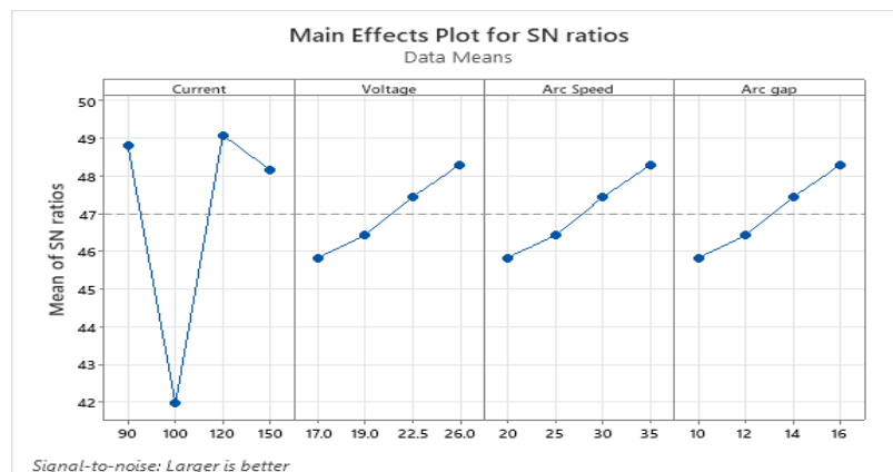
Figure 4.6 Main effect plot for S/N ratios for Tensile Strength.
