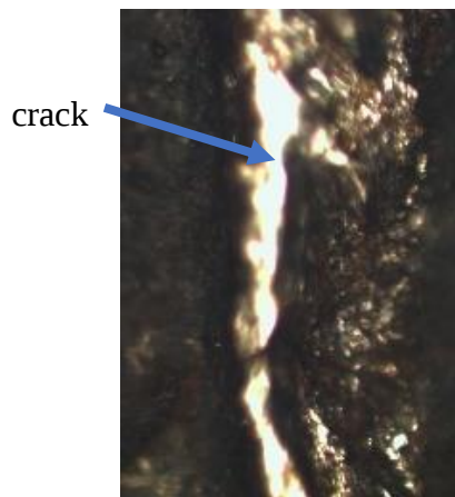
Figure 4.2 crack analysis during microscopy at ASTU material science lab
