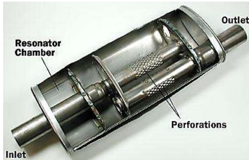
Figure 1. Cut way View of a Conventional Muffler
