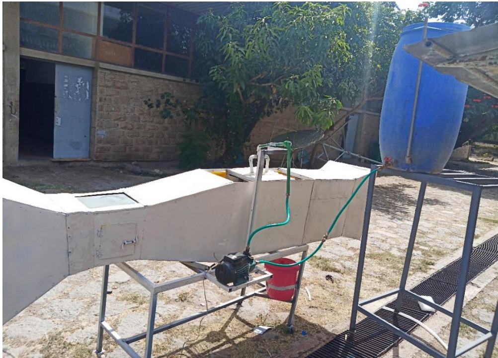
Figure 5. 11: Experimental setup of the central liquid based air filtration system.
