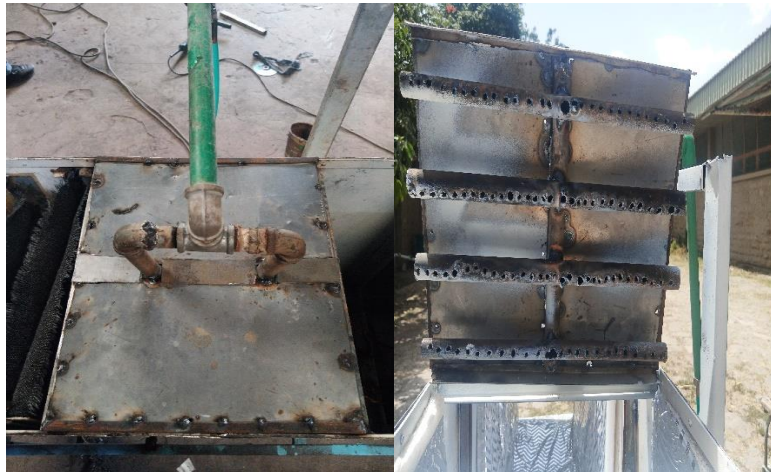
Figure 5. 8: Water distribution header
