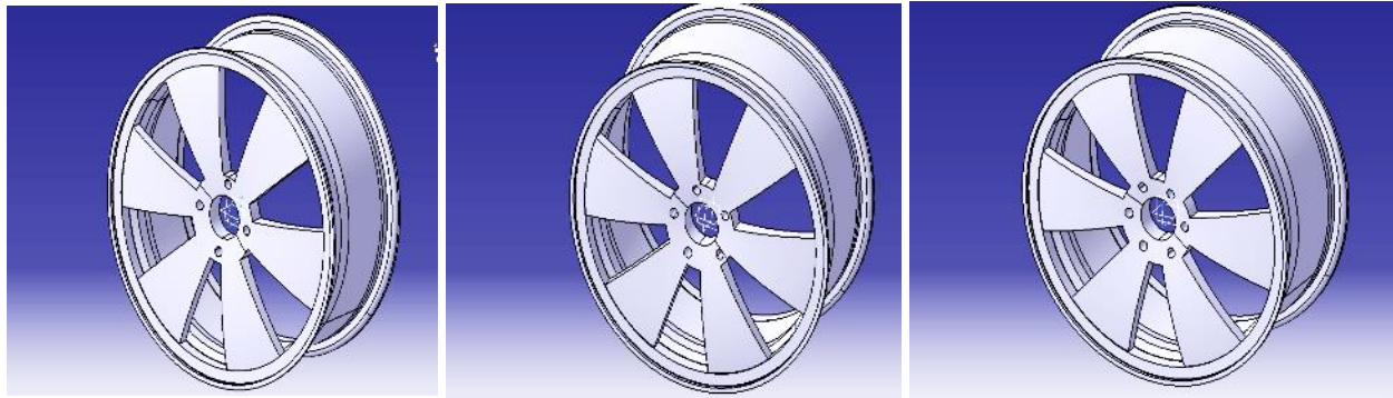
Figure 4.3: wheel rim design of 4, 5 and 6 bolt holes with six spokes
