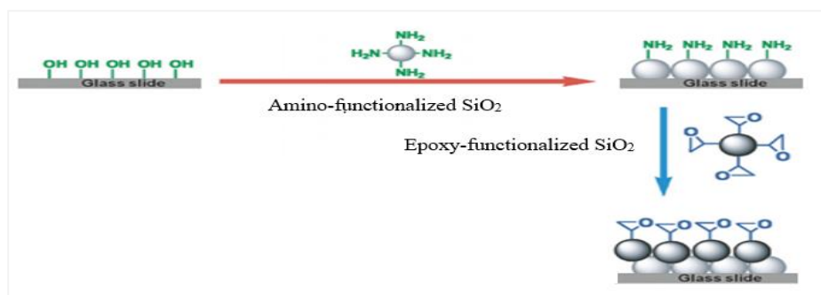
Figure 2.14 Schematic illustration of preparation of superhydrophobic surfaces on glass surfaces.
