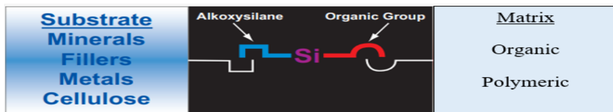
Figure 2.5 The bridge formation of an organosilane molecules.
