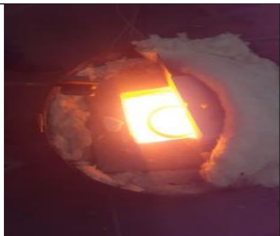
Stir cast melting of bar
