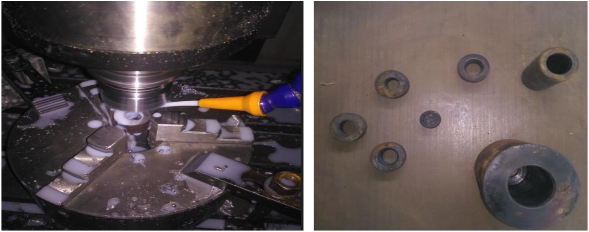
Figure 3.23 Die design and fabrication
