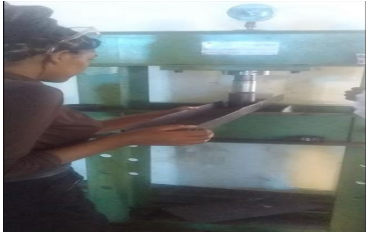
.Figure 3.24 Cold deforming using hydraulic pressure
