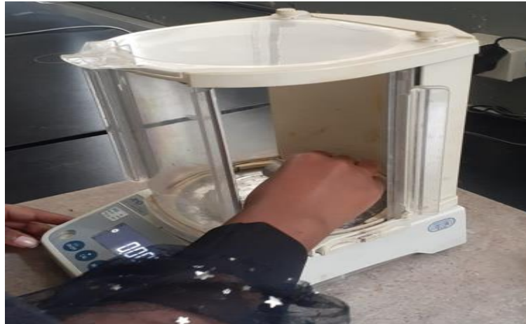
Figure 3.13 Measuring the mass of developed composite using Analytical precision balance
