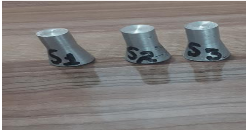
Figure 4.19 Cold extruded samples
