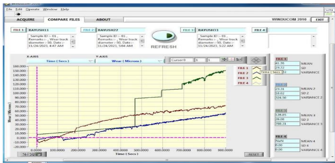
Figure 4: 4 wear rate verses time for sample 1, 2,3
