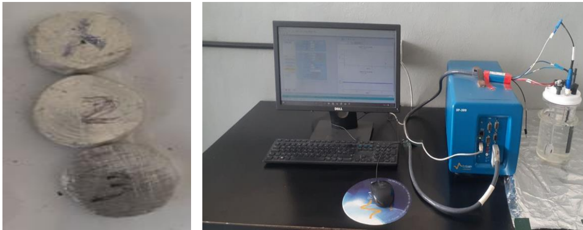
Figure 3.18 Corrosion on developed composite in 3%NaCl Electrochemical Analyzer
