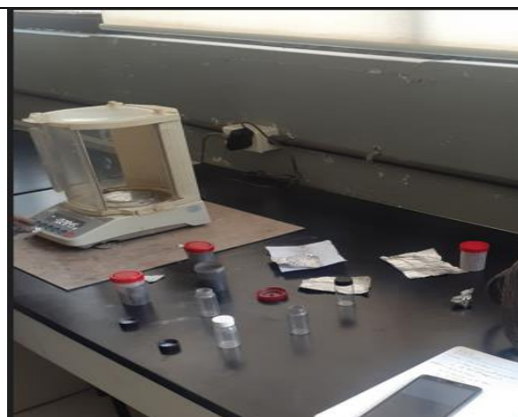
Measuring the reinforcement weight
