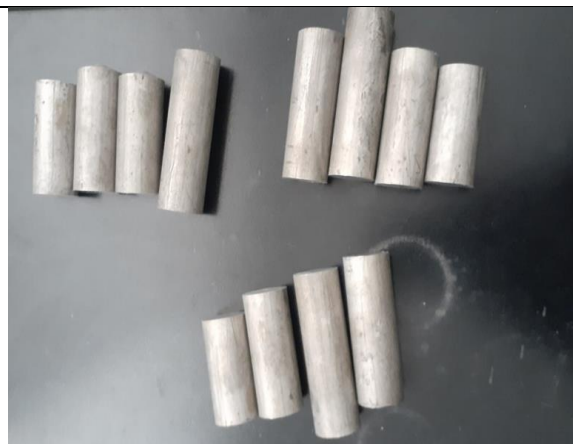
Chopped bar of 7075 aluminum bar
