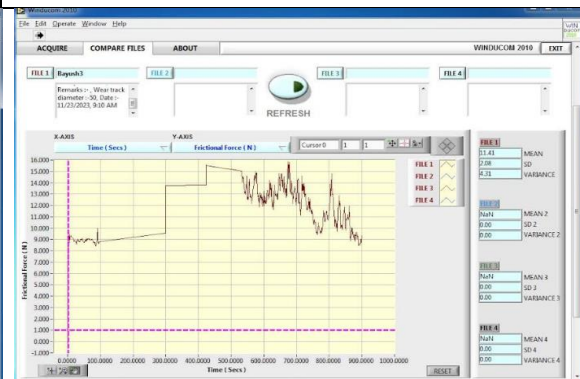
Friction force verses ime for sample three
