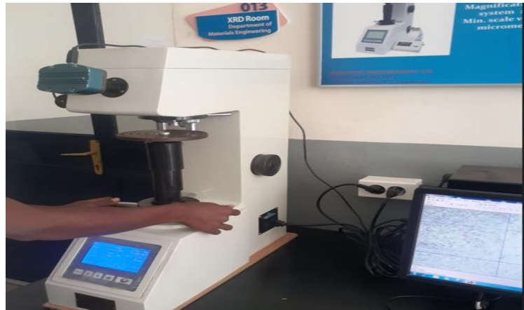
Figure 3.15 Measuring the hardness developed composite
