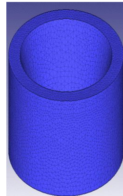
Figure 3.19 Material defining and meshed parts in preprocessors level
