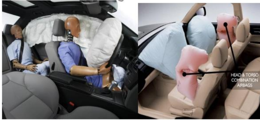
Figure 2. 1 Side safety airbag system (Arun Kumar & Madhu, 2015)
