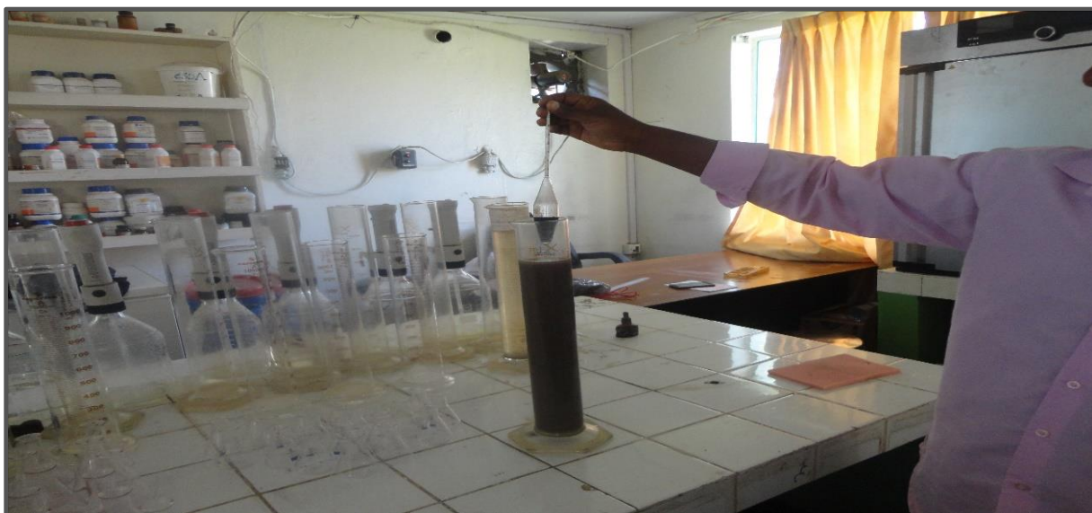
Figure 3.5: Graduated cylinder (1000ml) and hydrometer ( \text{g liter}^{-1} or percent)
