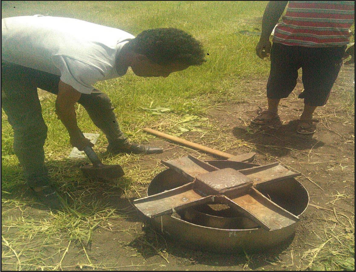
Figure 3.6: Double ring infiltrometer at the field 135
