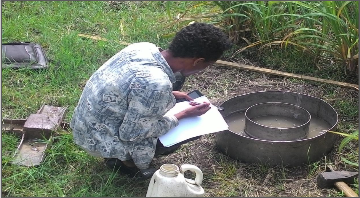
Figure 3.7: Time interval and infiltration rate records
