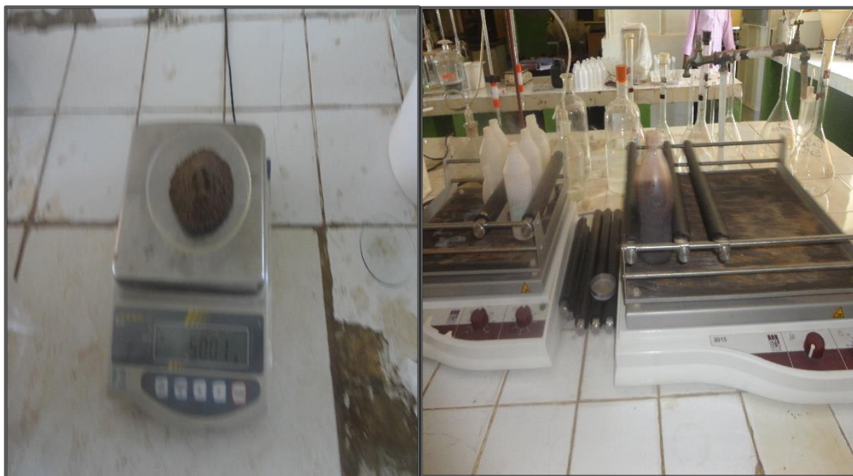
Figure 3.4: 50 gram of soil and oscillatory shaker
