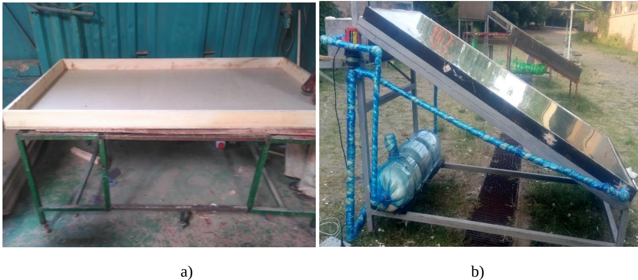
Fig 6.6 Photograph of collector a) wooden casing with back thermo-foam insulation and b) FPC with cover glass
