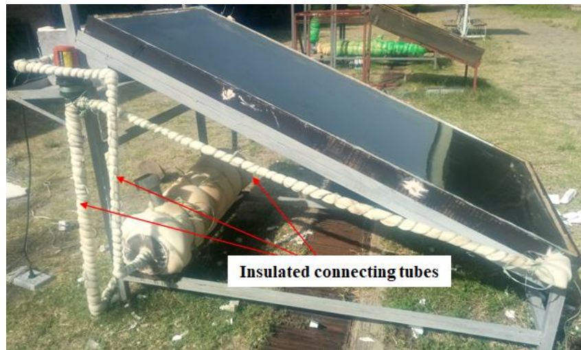
Fig 6.12 Connecting tubes of closed the loop
