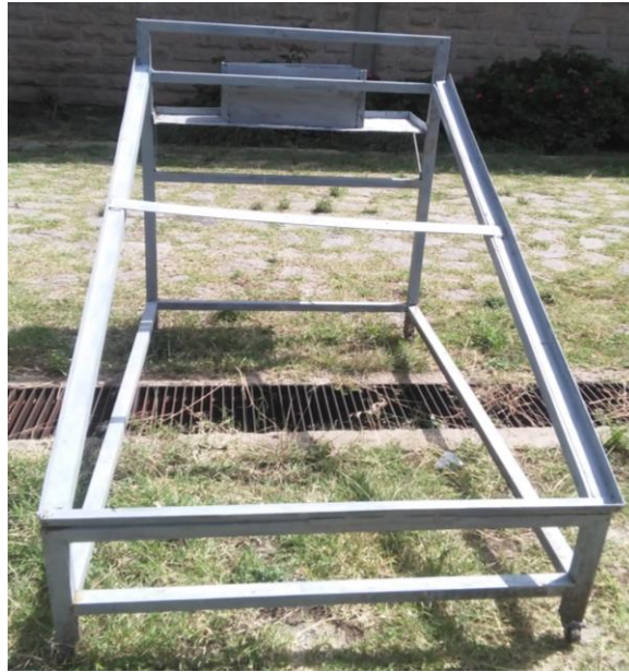
Fig 6.3 Supporting frame and structure of the prototype
