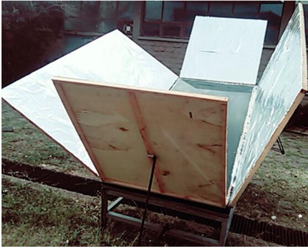
Fig 6.7 Collector with four reflectors in all the sides
