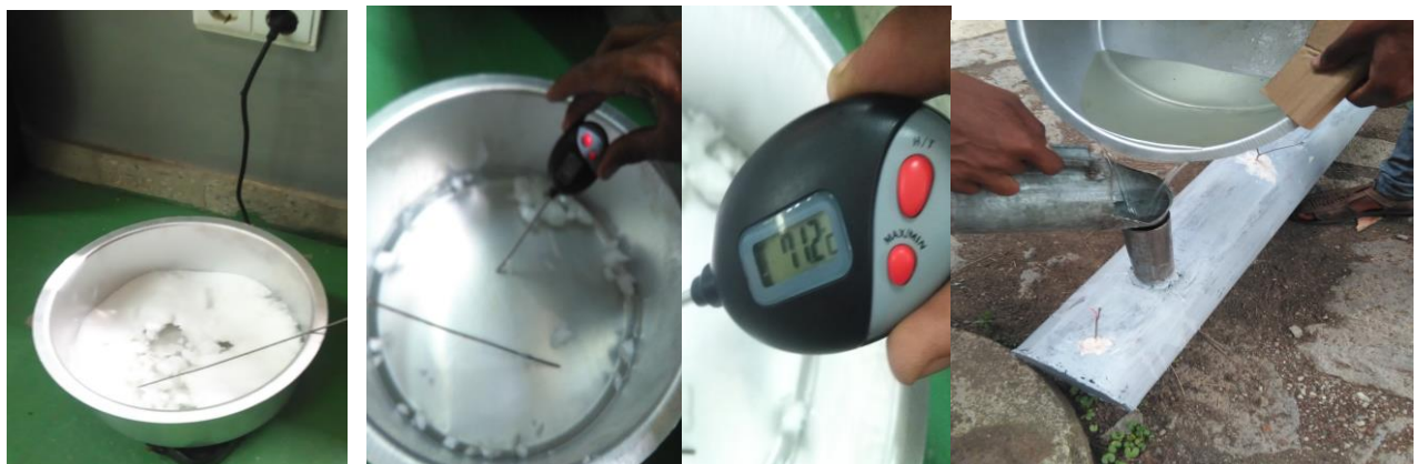
Fig 6.13 Melting and pouring process of stearic acid in to shell and tube storage unit.
