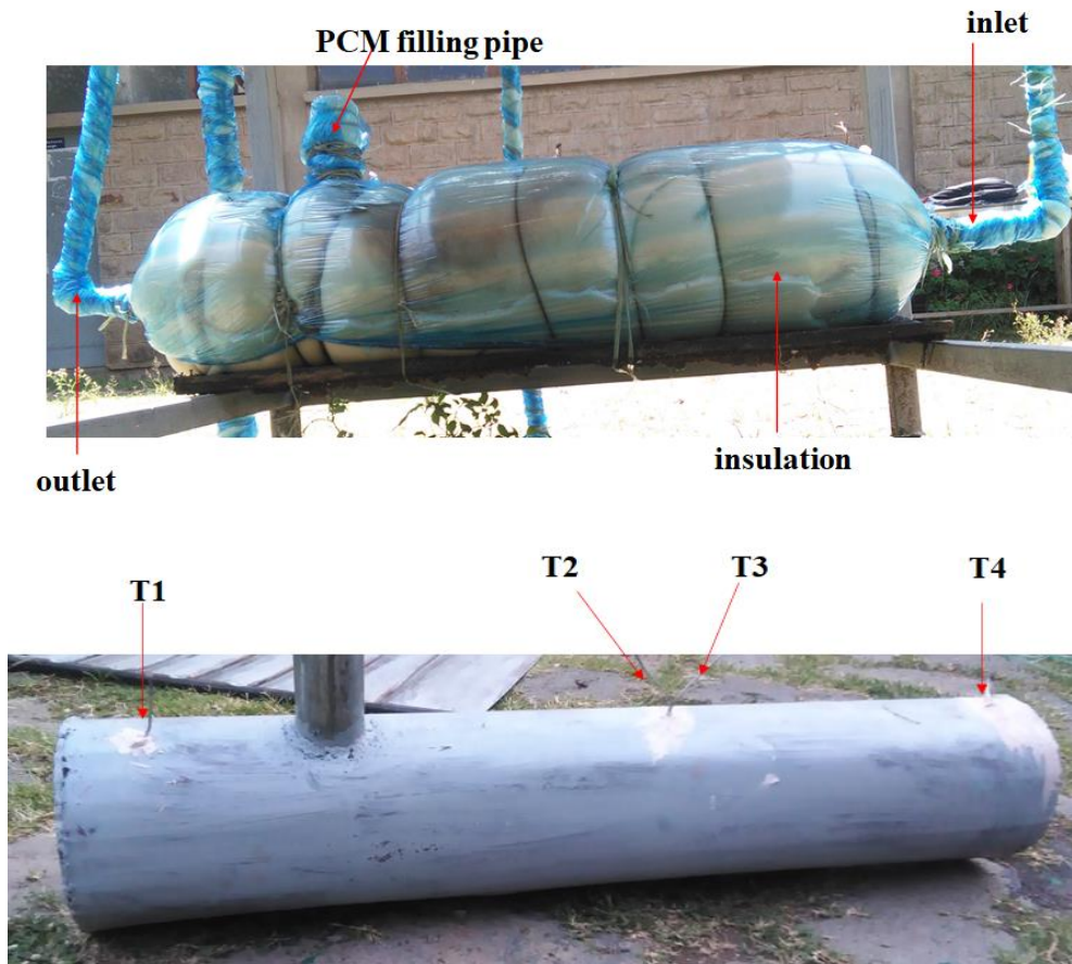
Fig 6.14 Setup of LHS unit and positions of thermocouples
