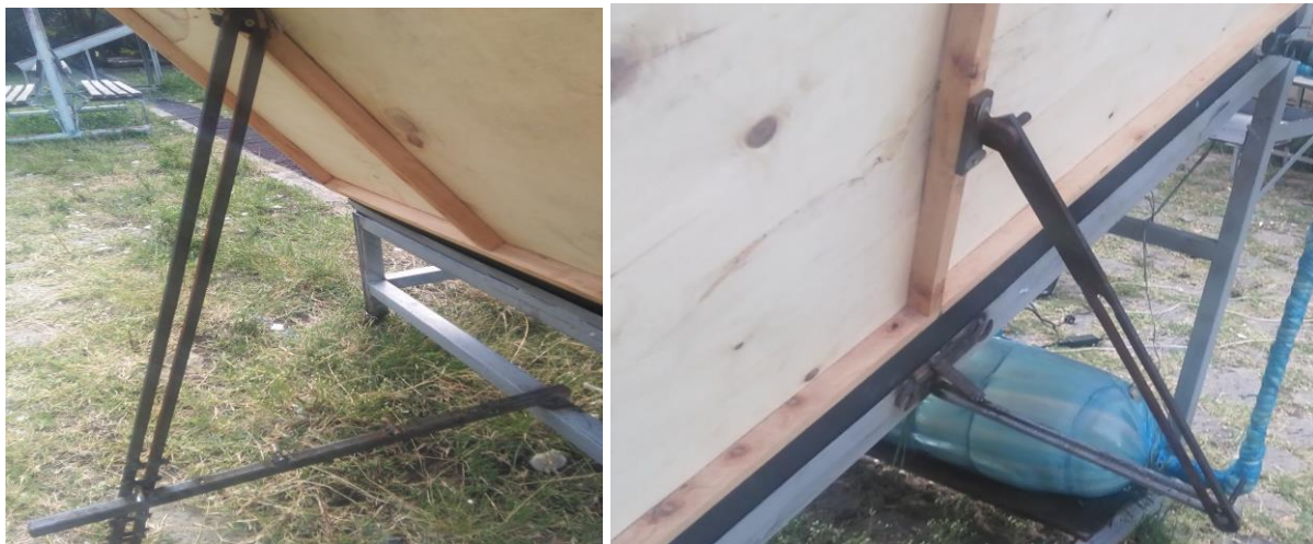
Fig 6.8 Manual adjusting mechanism for the reflectors
