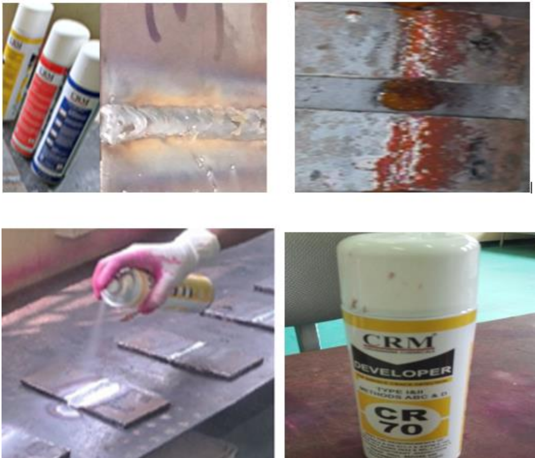
Figure 3. 8 . a) PT process pre cleaning sample by using general purpose cleaner, (b)application of developer, (c)inspection pent surface and (d) cleaning anti-corrosion solution
