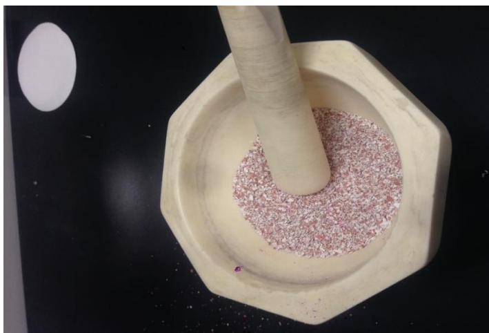
Figure 3-3: crushing the cleaned egg shell for calcination
