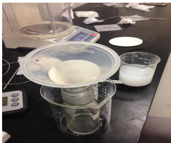
Figure 3-6: filtering using filter paper the final precipitates
