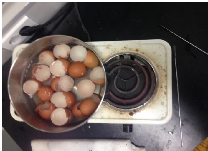
Figure 3-2: Egg shells being cleaned using boiling water
