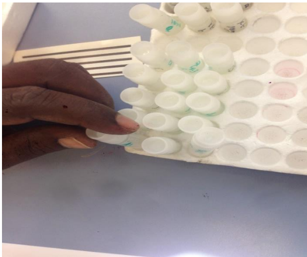
Figure 3-8: Sample prepared with a serial dilution from HA powder samples
