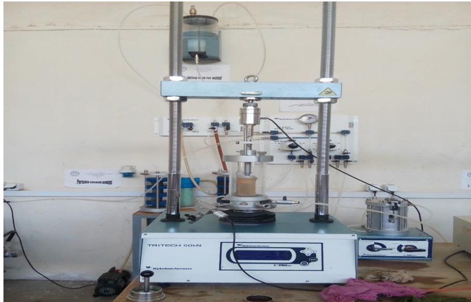
Figure 3.6: Tri-axial machine used for this study
