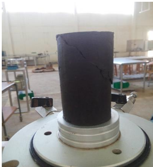
Fig C-3: sample after shearing
