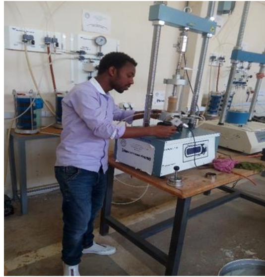
Fig C-2: Mounting sample on tri-axial machine
