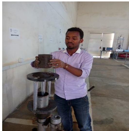
Fig C-4: when extruding sample from mold
