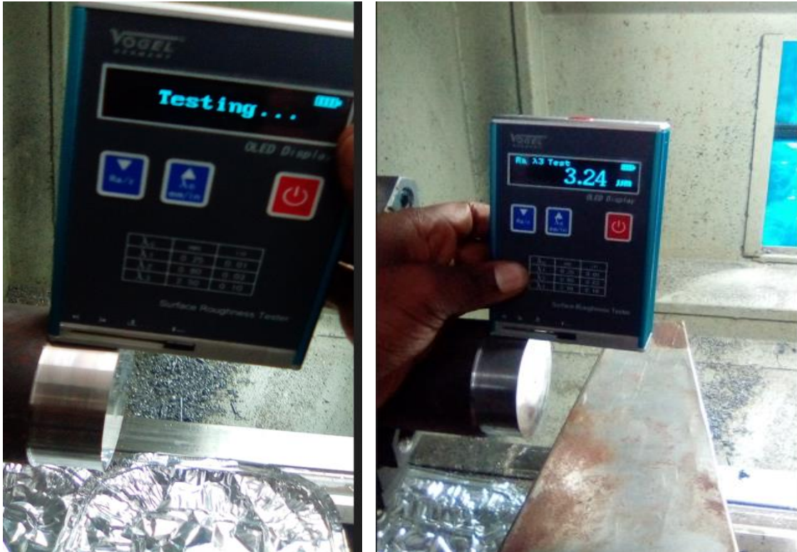
Figure 4. 10 Surface Roughness At 90 m/min, 0.5 mm, And 0.15 mm/rev.
