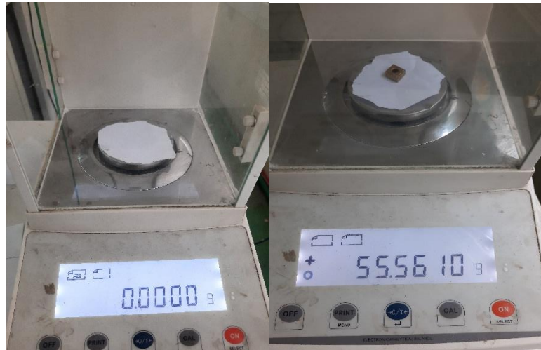
Figure 3. 10 Digital Balance to Measure Weight Loss of Cutting Tool Insert
