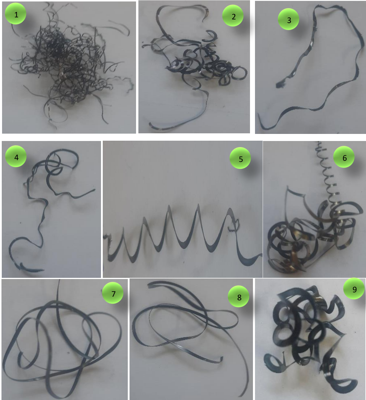
Figure 4. 47 Chip Formed During Turning AISI 1030 Steel Experiments
