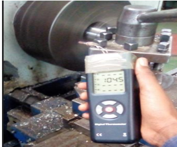
Figure 4. 19 Tool Temperature at 170 m/min, 0.5 mm, And 0.25 mm/rev.
