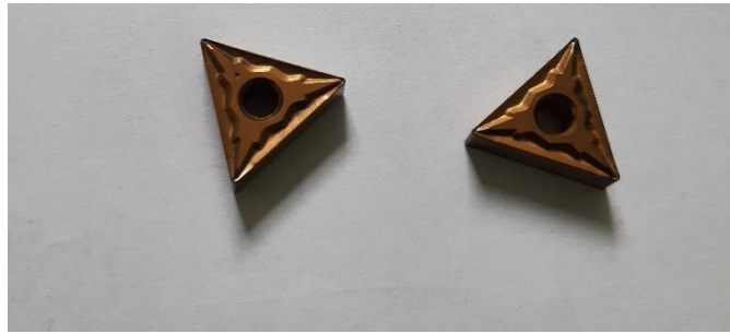
Figure 3.14 Tungsten Carbide Cutting Tool for Wear Calibration
