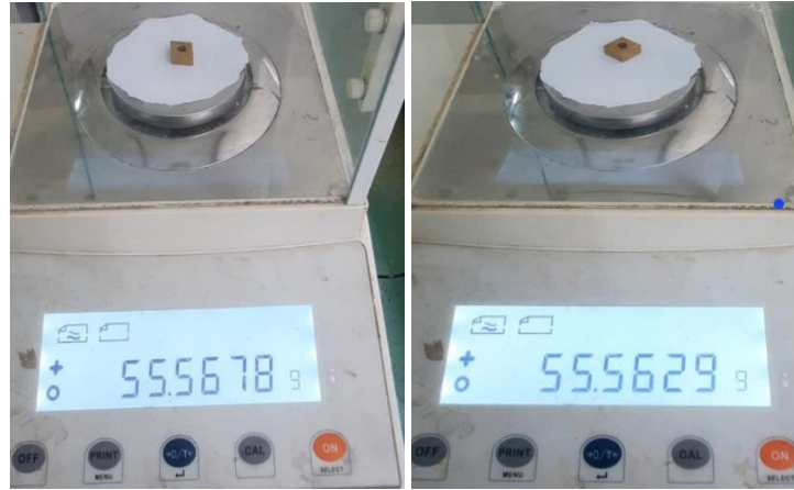
Figure 4. 32 Weight Loss of Insert at 90 m/min, 0.5 mm, and 0.15 mm/rev (Exp. 1)
