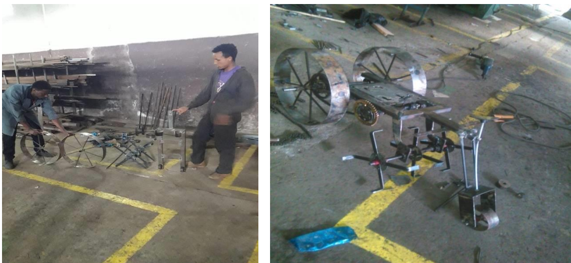
Fig.3.20. Fabrication of motorized rotary weeder component in AAERC workshop.
