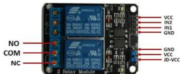
Figure 13. Relay module pin out
