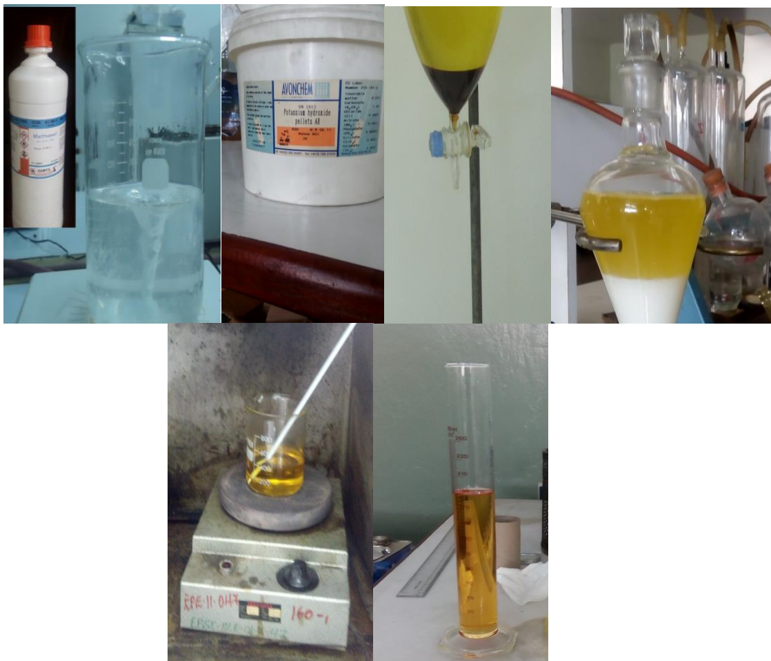
Figure 6 Transesterification and washing process
