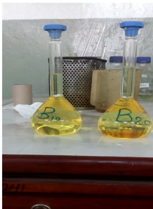
Figure 7 Preparing blends of biodiesel
