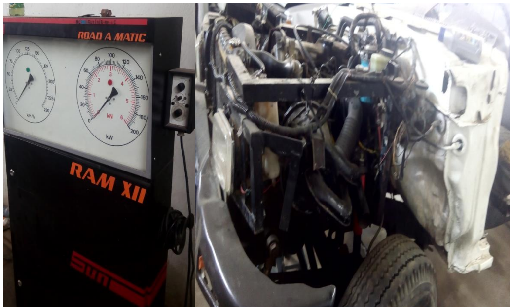
Figure 12 Chassis dynamometer for vehicle (engine) performance testing
