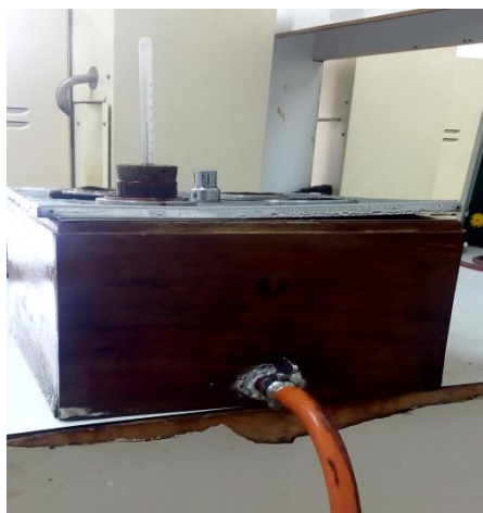
Figure 10 Cloud point measuring apparatus
