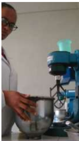
Mortar under mixing
