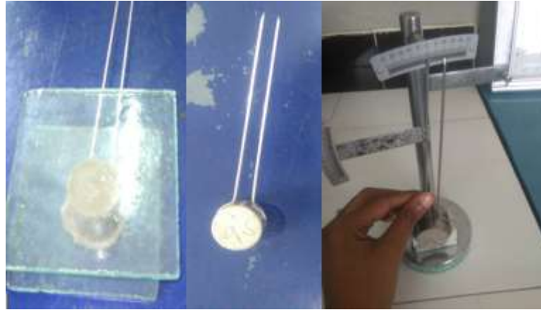
Figure 3.12 Le-Chatelier Expansion Measurements
