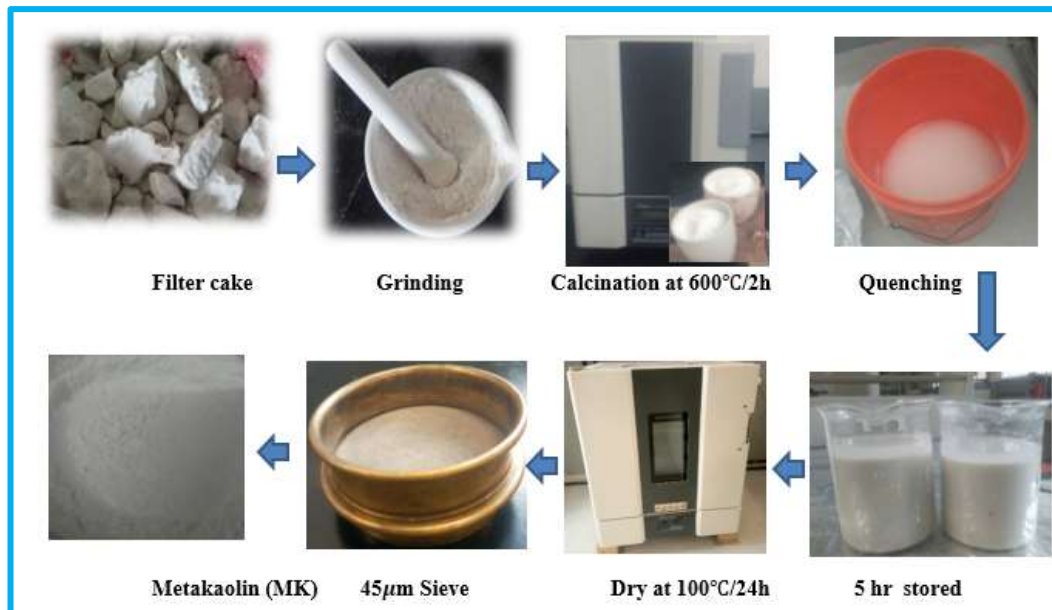
Figure 3.2. Metakaolin materials preparation from the filter cake.
