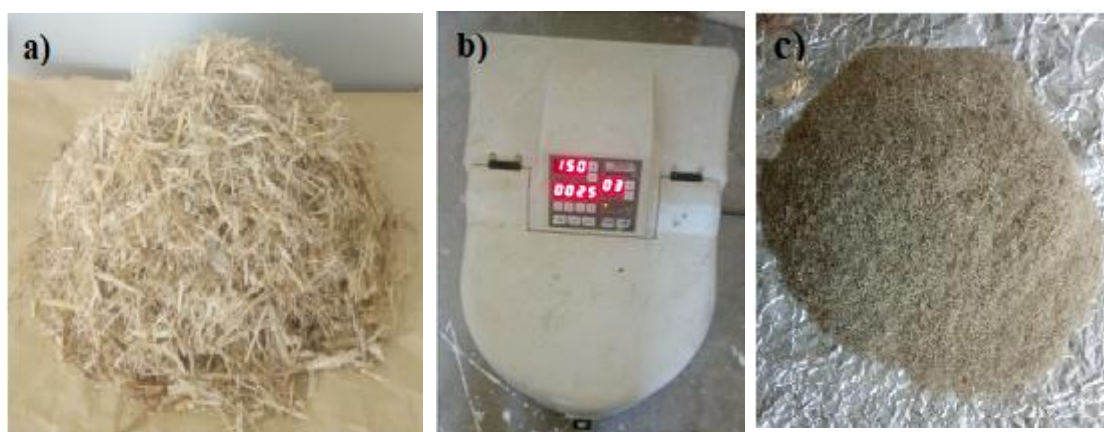
Figure 3.2 a) Sugarcane bagasse before size reduction; b) Size reduction of sugarcane bagasse using Ball mill at 150rpm; c) Sample after size reduction
