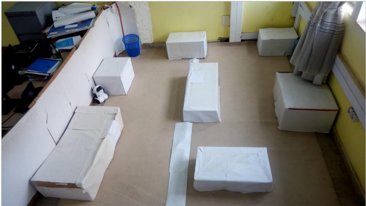
Figure 5.2 Test-bed for Mobile Robot Indoor Navigation
