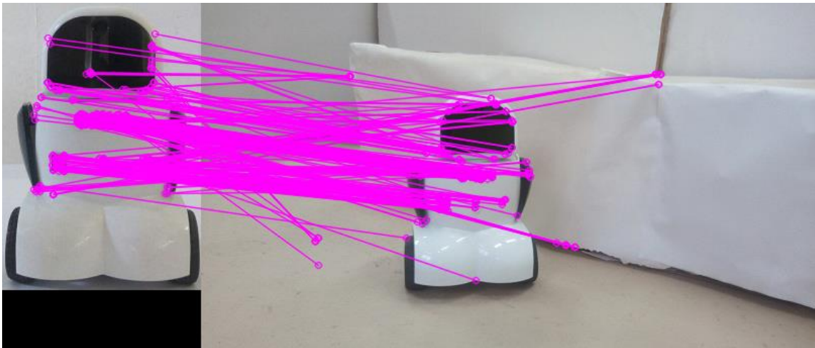
Figure 6.10 Feature Matching Sample Using ORB+SURF and FLANN
