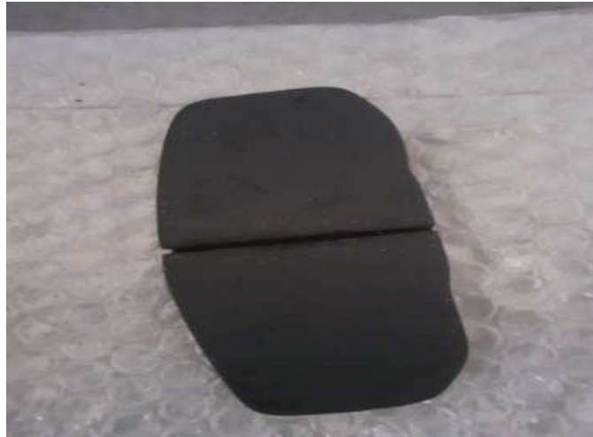
Figure 4.16: Developed composite brake pad
