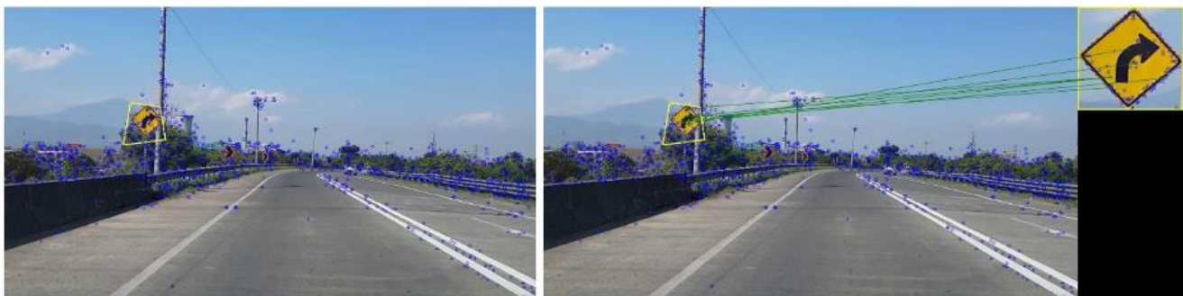
Figure3.19Detecting road side sign for curved road (S H Supangkat 2018)
