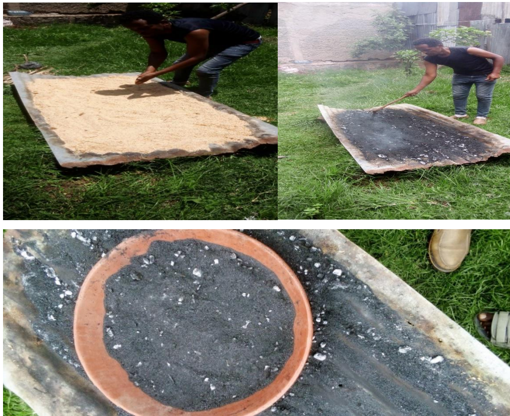
Figure 3.3 Process of saw dust ash (SDA) sample preparation
