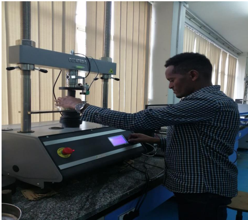
Figure 3. 4 photographic view of UCS test
