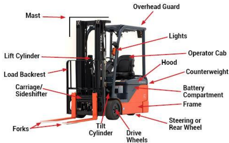
Figure 1.3: Various components of Toyota electric forklift (Summit Toyotalift, 2023)
