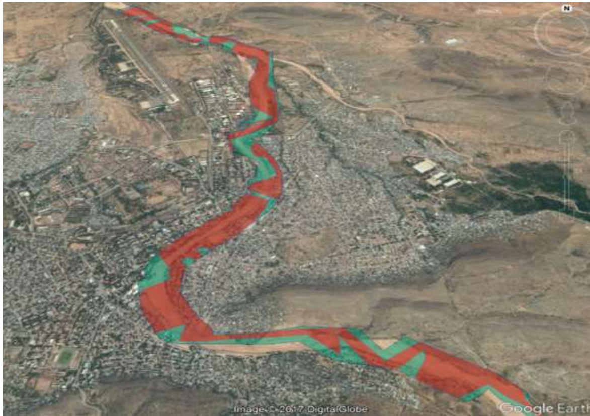
Figure 4.14 Flood Inundation map superimpose on Google earth for 5 year (red) and 100 year (green) return period.
