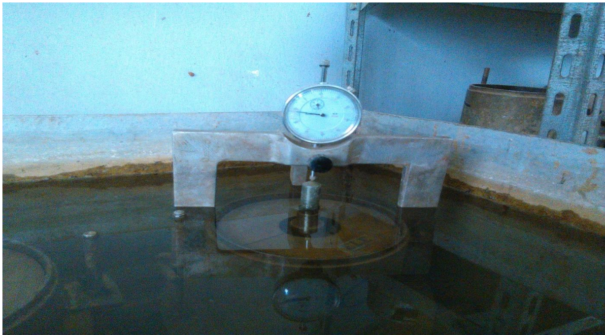
Fig.5.5 photo of soaked soil mold for CBR test
