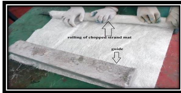
Figure 3.8 Rolling method of chopped strand mat
