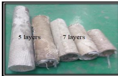
Figure 3.17 Products of PWR pipe
