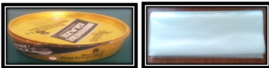
Figure 3.26 Releasing wax gelcoat and plastic sheet film
