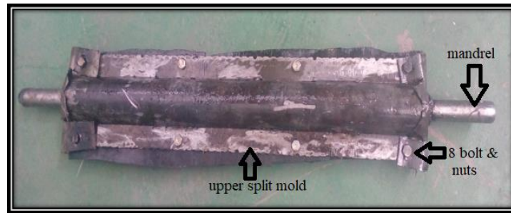
Figure 3.14 Assembly of mold manufacturing
