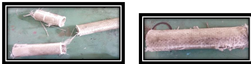
Figure 3.15 First product of GRP pipe
