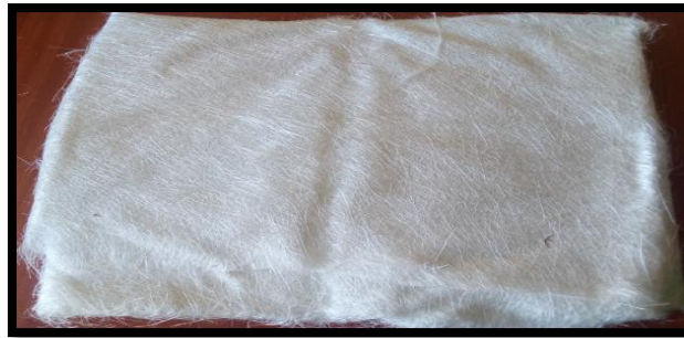
Figure 3.1 Chopped strand mat layers.
