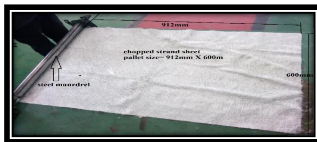
Figure 3.7 Mandrel seat over chopped strand mat
