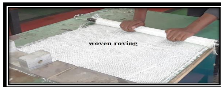
Figure 3.9 Rolling of woven roving
