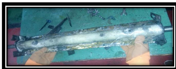
Figure 3.13 demolding the product by removing half split mold.
