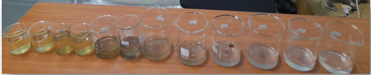
Figure A1: treated fluoride containing water with bone char prepared at 450°C-800°C, each of the temperature set points; 1 and 2 h
