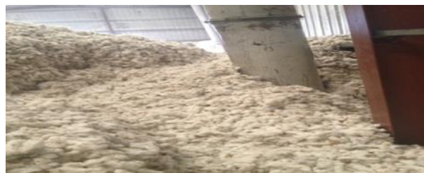
Figure.4. 9. Seed cotton preparation for removal of sand
