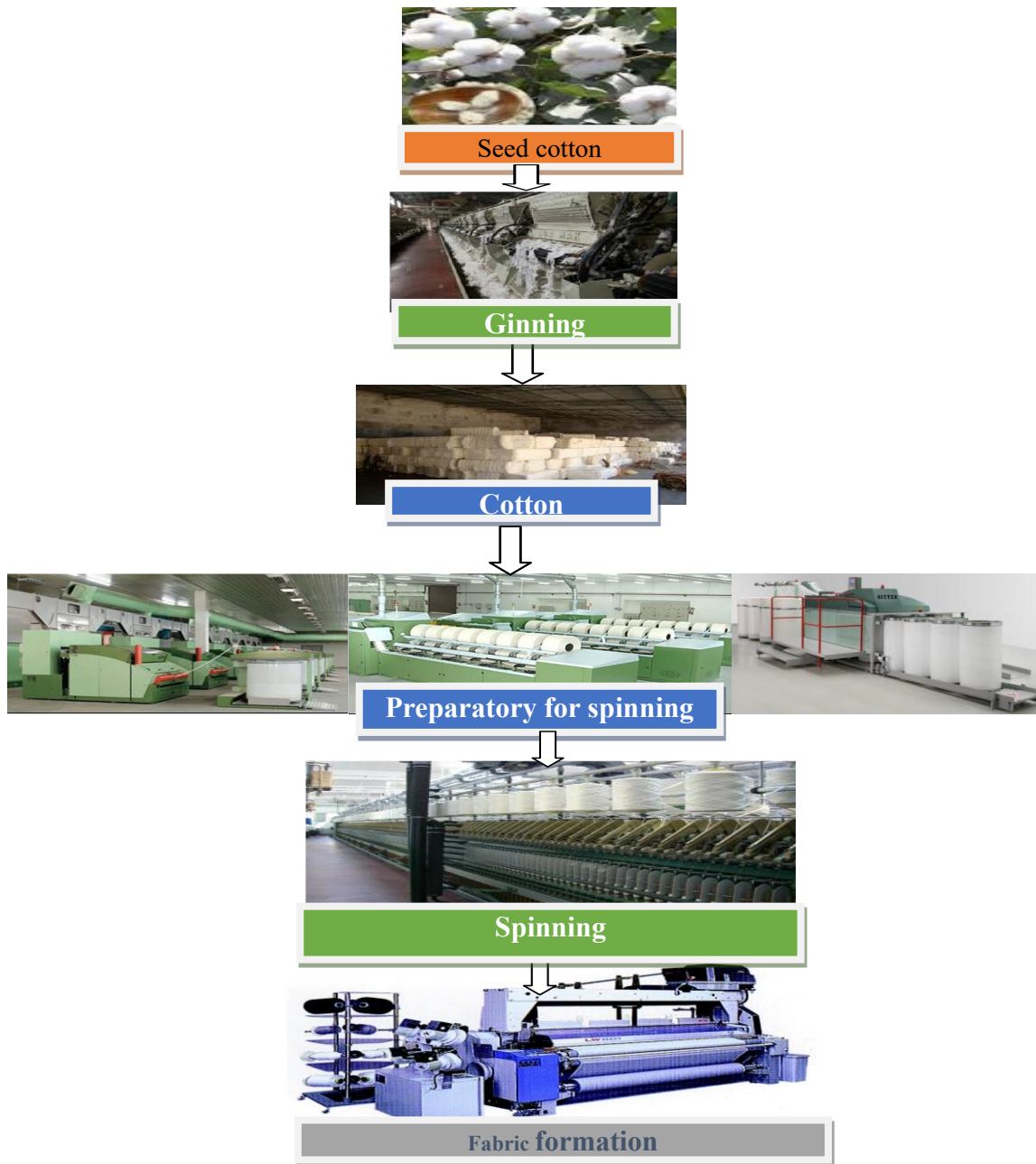
Figure.3. 1.Sequence of operation in textile process
