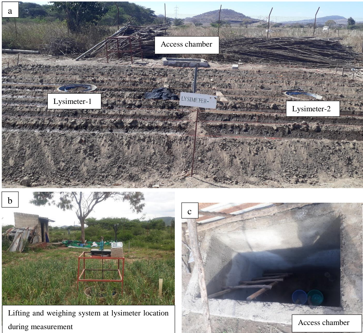
Figure 4-5. Lysimeters with access chamber (a), lifting and weighing systems (b), and inside of the access chamber (c)
