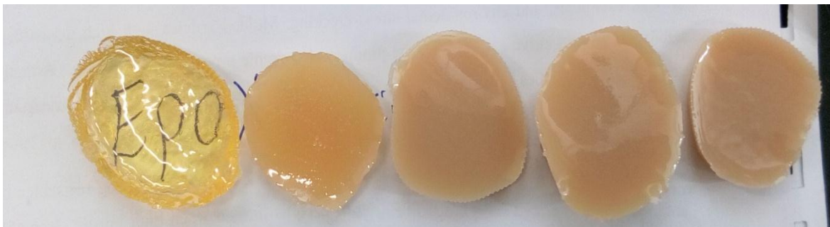
Figure 3.7. The reduction in transparency due to the addition of MK filler
