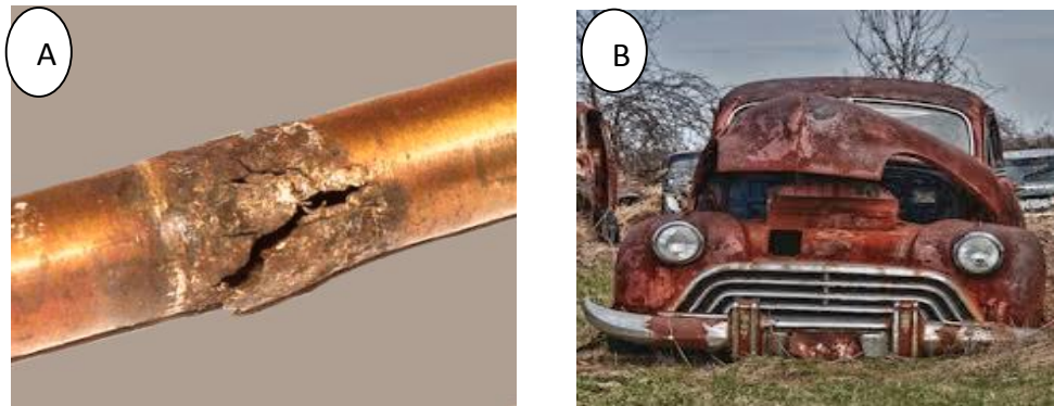
Figure 2.1. Corrosion and its impact on A) metal pipe and B) automobile car
