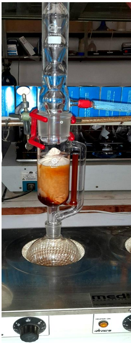
Figure 3.2: Visibility of layers in soxhlet extraction acetone solvent (A.M.C.F)
