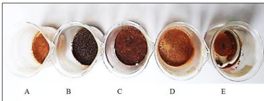
Figure 4.3: The dried residue of Acetone (A), Acetonitrile (B), Ethyl acetate (C), and Methanol (D) and Solvent mixture (E) extraction obtained after separation.
