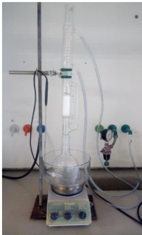
Figure 3.1: Experimental set up of Soxhlet solvent extraction (Dreamstime.com https://www.dreamstime.com/soxhlet... )
