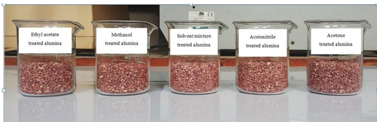
Figure 4.2: Soxhlet extraction solvent treated alumina
