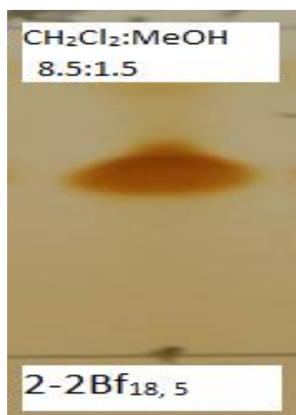
Figure 7: TLC profile of the compound-2
