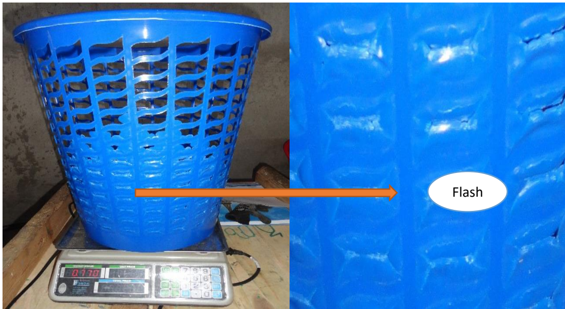
Figure 4.1 Flash defect on laundry bucket.
