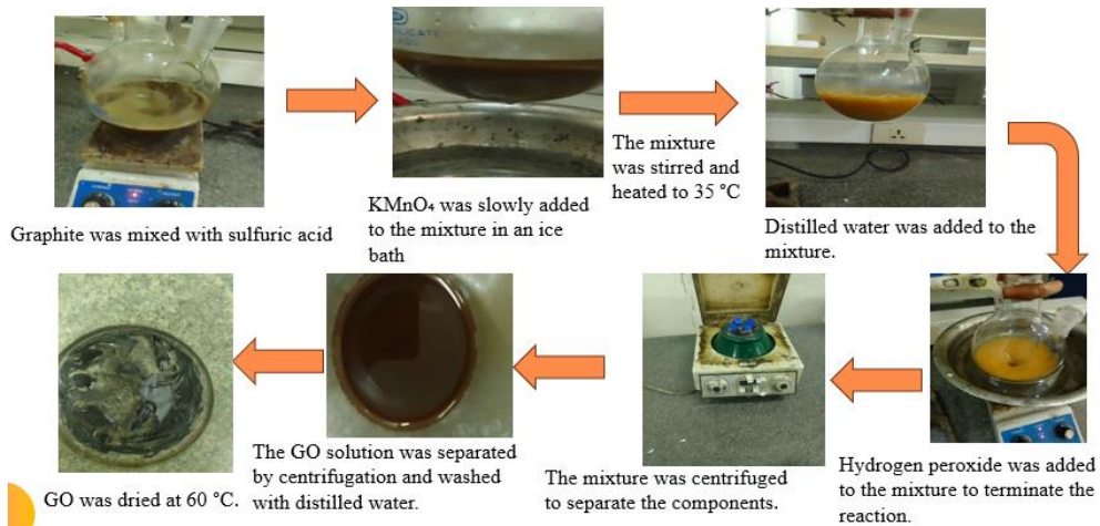
Figure 7. 2. Synthesis graphene oxide (GO) by modified Hummers' method
