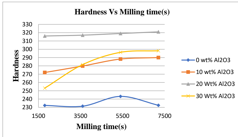
Figure 4.7 Graph of hardness versus milling time
