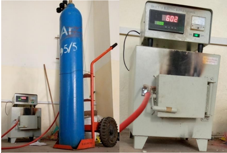
Figure D-7 a) the sintering arrangement with gas cylinder fig b) furnace at 600°C on sintering process.
