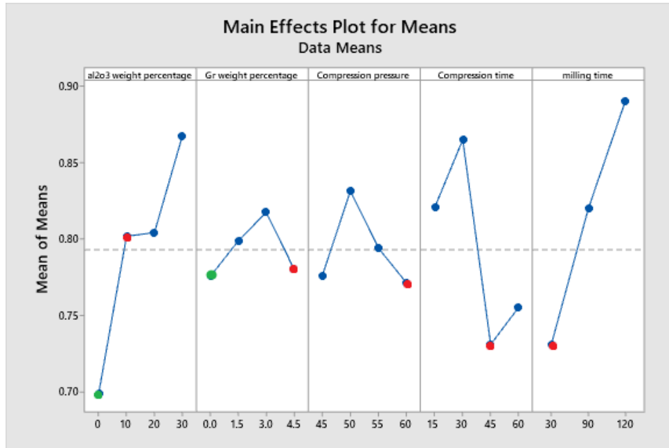
Figure 4.34 main effect plots for means of GRG of actual density, porosity
