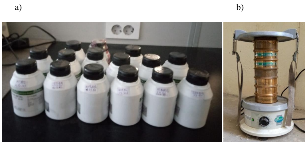
Figure D-6 a) The powder re stored inn to plastic jar after milling process. fig b) Shaker (armfield CEN-MVII-00A) utilized for sewing purpose.
