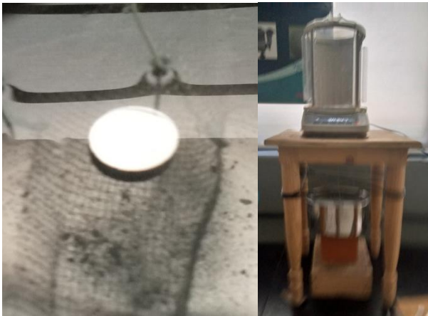
Figure D-8 a) Sample being submerged in water and weighed. Fig b) Arrangement for weight measurement in water.
