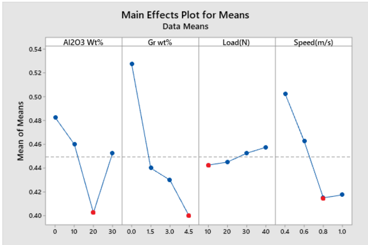
Figure 4.33 Main effect plots for means of CoF.
