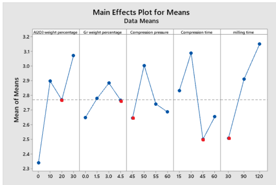
Figure 4.3 Main effect plots for means of porosity
