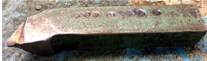
Figure 3-5 Cemented carbide tool
