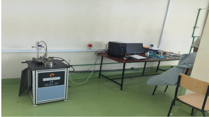
Figure 3-8 Taylor and Hobson profilometer used to measure surface roughness (AASTU, Department of Material Engineering )
