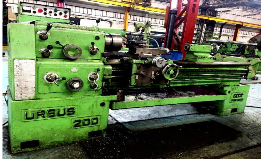
Figure 3-2 Conventional lathe machine, URUSUS 200 model
