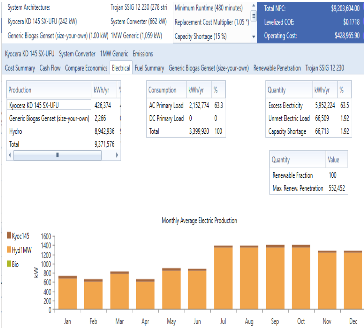
Figure 4.14 Electrical properties of standalone hybrid system from the 1 st case
