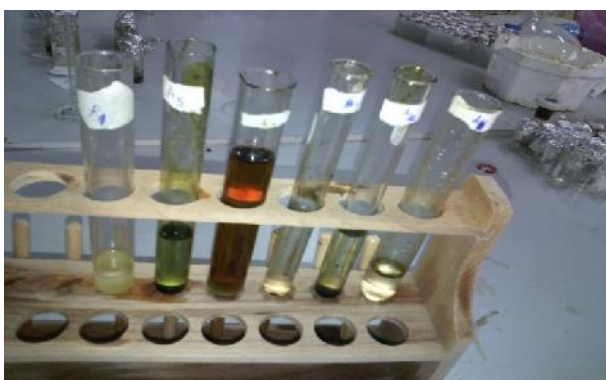
Fig 18 Results for flavonoid test from left to right \text{R}_1^+ , \text{A}_5^- , \text{A}_4^- , \text{A}_1^+ , \text{A}_2^+ , \text{A}_3^+
