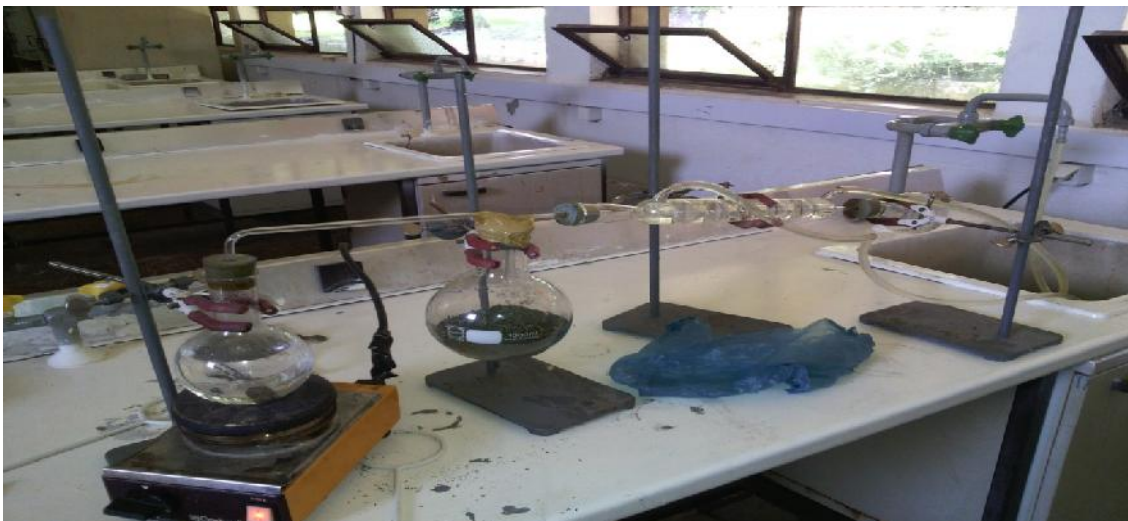
Fig.16 The set up of steam distillation(Adama,ASTU)
