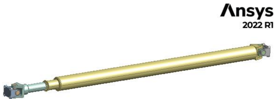
Figure 4.12: The Geometry of the existing shaft after imported to ANSYS
