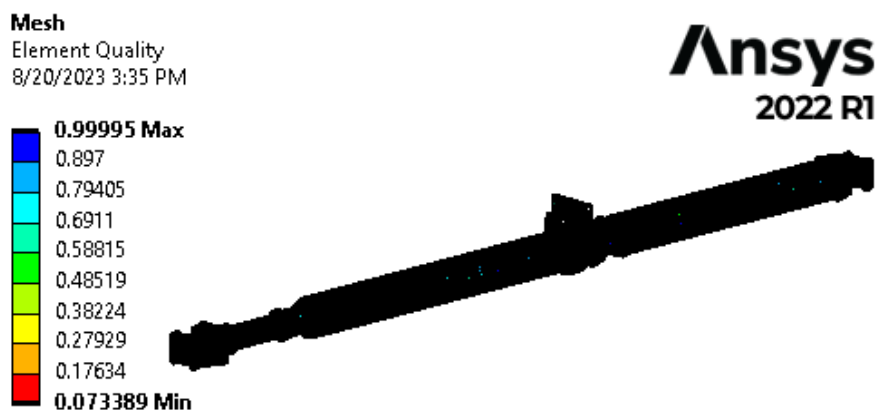
Figure 4.18: The quality of the generated mesh for the existing assembly
