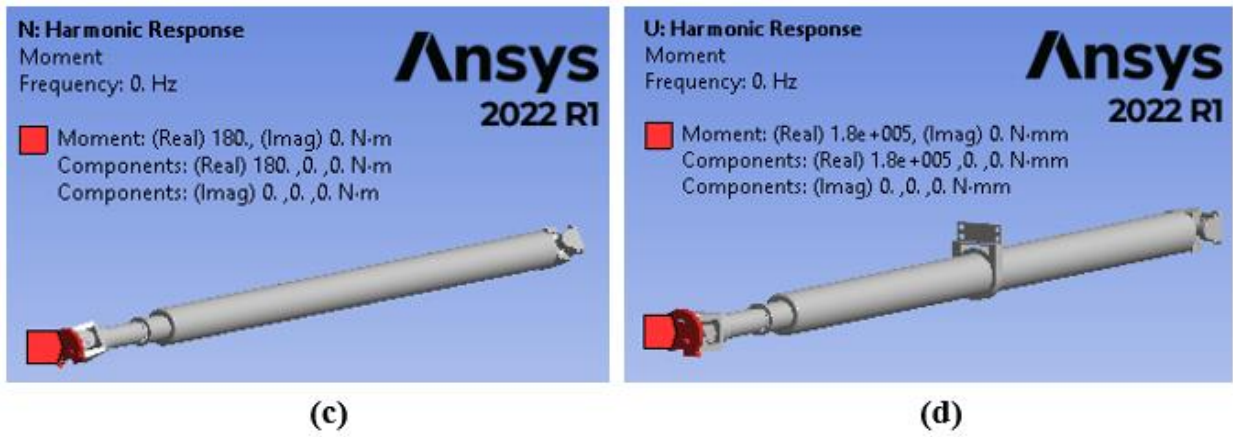
Figure 5.31: Applied load for (a) the existing model (b) two-piece modified model (c) one-piece modified model without center bearing (d) one-piece modified model with center bearing
